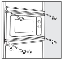
Secure the appliance to the side walls of the unit with screws (A). Then press cover caps (B) onto the screws.
